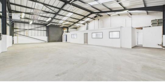
The subjects comprise an end terraced industrial unit which is laid out to provide warehouse, office, W.C, kitchen and yard/car parking. The unit is of a steel portal frame construction with blockworks walls externally rendered to the lower sections with the upper sections being clad in profile metal sheeting. The roof over is pitched and similarly clad incorporating a number of translucent roof panels.
